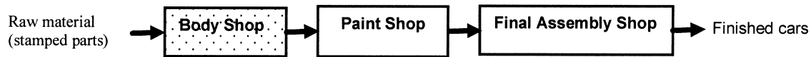
Figure 1: The body shop is at the upstream end of the work flow in a typical car plant.
